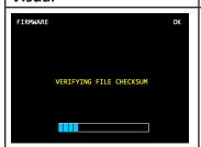
Before the tester reboots, it first checks if the newly installed files can be found. This takes max. 2 minutes.
